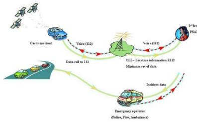
to the closest 112 PSAP sending a data message that uses common European standards. The EC set the eCall requirement for all new vehicles until 1<sup>st</sup> October 2017. Still, today no full integration of eCall modules has been accomplished in PSAP environments.
