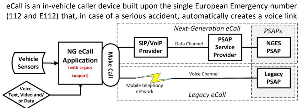
The eCall concept is currently deployed based on circuit switched emergency calls, specifically for 2G and 3G networks using an in-band modem. As next generation Emergency Services evolve towards a 4G communications framework, the eCall concept will be adapted as an IMS emergency call (current proposed solution for the eCall interface is SIP), hence benefiting from the resource efficient packet based systems.
